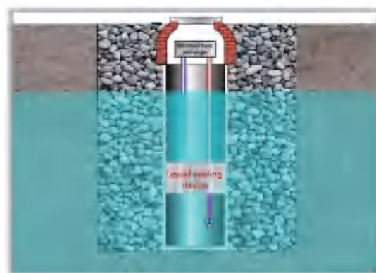
Fig.2 Geothermal Energy Collection Well With Heat Exchange Particles
